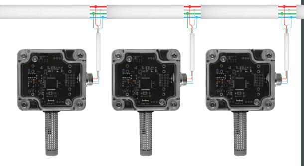
For the ease of installation and maintenance, the wires of the address line and the supply voltage are connected to the patch panel terminal blocks. Next an addressable controller is installed into the panel
