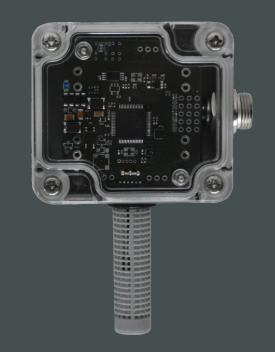
The multisensor recorder is a plastic body with a connector, an air intake probe and a transparent top cover allowing to determine the particulate level in the measuring chamber. The recorder body also includes the forced air intake system, measuring modules, LED indicator, power supply and a microcontroller
