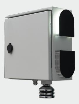
The station metal casing encloses a measuring module, a power supply, a microcontroller and a GSM / NBIoT modem. It supports connection up to 30 additional external measuring elements. The data exchange and accessary power supply is carried out via the 4-wire address line with a length of up to 1,000 m
