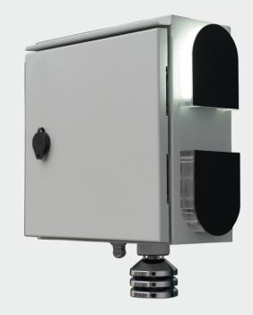
The station metal casing encloses a measuring module, a power supply, a microcontroller and a GSM / NBIOT modem. It supports connection up to 30 additional external measuring elements. The data exchange and accessary power supply is carried out via the 4-wire address line with a length of up to 1,000 m
